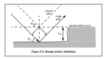
where  $S_{state}$  is the sea state, which is tabulated in several cited references. The sea state is characterized by the wave height, period, length, particle velocity, and wind velocity. For example,  $S_{state} = 3$  refers to a moderate sea state, in which the wave height is approximately 0.9144 to 1.2192 m, the wave period 6.5 to 4.5 seconds, wave length 1.9812 to 33.528 m, wave velocity 20.372 to 25.928 Km/hr, and wind velocity 22.224 to 29.632 Km/hr.
