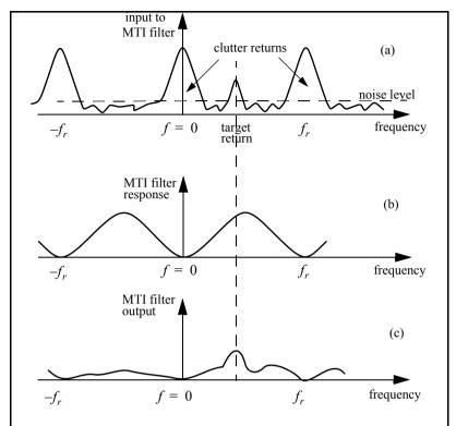
Figure 9.15. (a) Typical radar return PSD when clutter and target are present.
