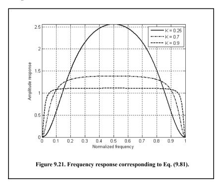
In order to avoid oscillation due to the positive feedback, the value of K should be less than unity. The value  $(1-K)^{-1}$  is normally equal to the number of pulses received from the target. For example, K=0.9 corresponds to ten pulses, while K=0.98 corresponds to about fifty pulses.
