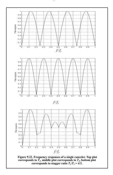
To better determine the frequency response of an MTI filter with staggered PRFs consider a three-pulse canceler with two PRFs, or equivalently two PRIs,  $T_1$  and  $T_2$ . In this case, the impulse response will be given by
