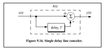
The delay T is equal to the radar PRI  $(1/f_r)$ . The output signal y(t) is
