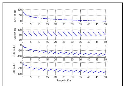
Figure 9.12. SIR, SCR, CNR, and SNR for a pulse Doppler radar with  $\sin(x)/x$  antenna pattern.
