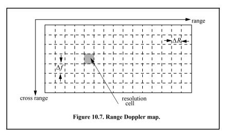
To further illustrate this concept, consider the case where  $N_a$  is the number of azimuth (Doppler) cells, and  $N_r$  is the number of range bins. Hence, the MAP is of size  $N_a \times N_r$ , where the columns refer to range bins and the rows refer to azimuth cells. For each transmitted pulse within the dwell, the echoes
