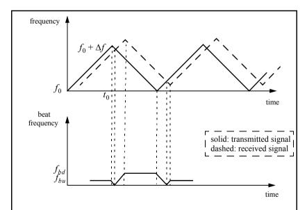
Figure 10.3. Transmitted and received LFM signals and beat frequency, for a moving target.
