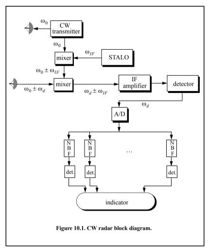
The NBF bank (Doppler filter bank) can be implemented using a Fast Fourier Transform (FFT). If the Doppler filter bank is implemented using an FFT of size  $N_{FFT}$ , and if the individual NBF bandwidth (FFT bin) is  $\Delta f$ , then the effective radar Doppler bandwidth is  $N_{FFT}\Delta f/2$ . The reason for the one-half factor is to account for both negative and positive Doppler shifts. The frequency resolution  $\Delta f$  is proportional to the inverse of the integration time.
