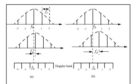
Figure 10.9. Spectra of transmitted and received waveforms, and Doppler bank. (a) Doppler is resolved. (b) Spectral lines have moved into the next Doppler filter. This results in an ambiguous Doppler measurement.
