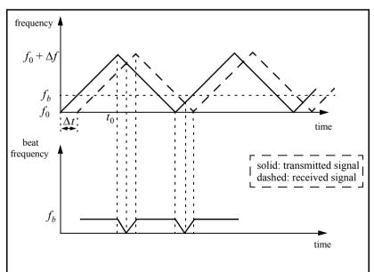
Figure 10.2. Transmitted and received triangular LFM signals and beat frequency for stationary target.
