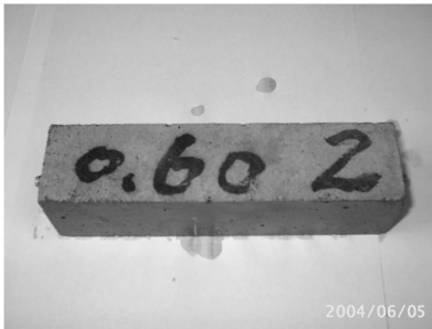
Fig. 1. Specimen of cement mortar with the w/c = 0.6 .
