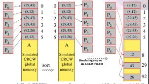
4. Each EREW processor  $P_i$  now inspects  $A[i]=(l_j,x_j)$  and  $A[i-I]=(l_k,x_k)$ , where j and k are values in the range  $0 \le j,k \le p-1$ . If  $l_j \ne l_k$  or i=0 then  $P_i$  writes the datum  $x_j$  to location  $l_j$  in the global memory. Otherwise, the processor does nothing.
