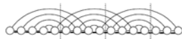
Inverting the mapping - mapping a 2D mesh into a linear array (congestion 5)
