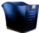
Each virtual processor is a hardware stream with its own instruction counter, register set, stream status word and target and trap registers. A different hardware stream is activated every clock period.
