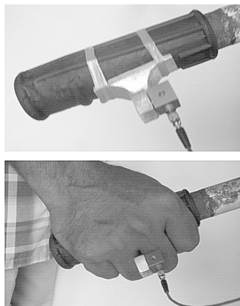
Figure 2 Mounting of accelerometer and hand adapter on existing handle grip of the hand tractor
