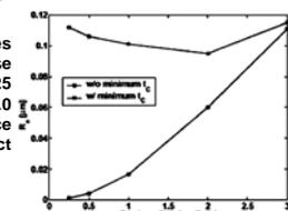
Comparing results of surface roughness with and without considering the minimum uncut chip thickness effect
