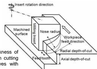
**Feed / tooth:** the thickness of chip material that each cutting edge of a tool removes with one pass.
