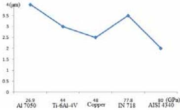
> No consistent concern between material shear modulus and MUCT.
